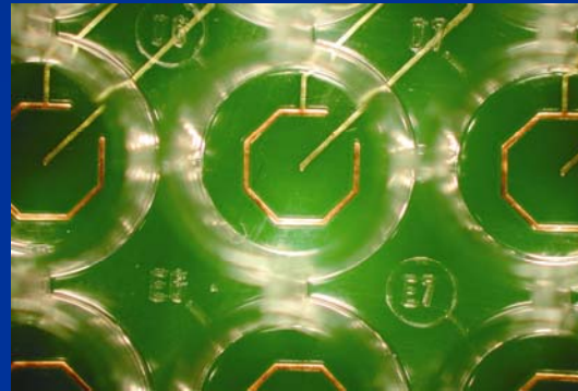
Electrodes in a 96-well QT-Screen plate from MultiChannelSystems
